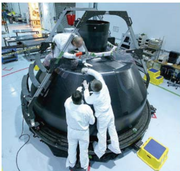
Pictured are fabricators at ATK in Iuka, MS laying up plies of composite material to create the inner honeycomb sandwich skin of the NASA crew module. The plies are being laid up with the assistance of a laser projection system (as indicated by the faint green lines on the top and side of the capsule), which is driven by FiberSIM software. With FiberSIM's Laser Projection module, engineers can automatically generate laser data files from within their CAD system directly from the 3D model of the composite part. This significantly increases engineering and manufacturing productivity, greatly reduces errors and makes updating and maintaining laser projection data easy.
