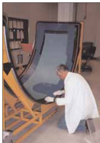
Layup of the inlet cowl upper skin repair.
