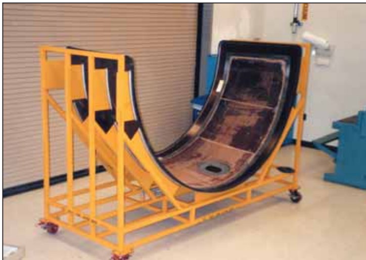
Boeing 757 inlet cowl upper skin with the inner facesheet removed for repair. The tool holds the part shape during layup and serves as the cure fixture.
