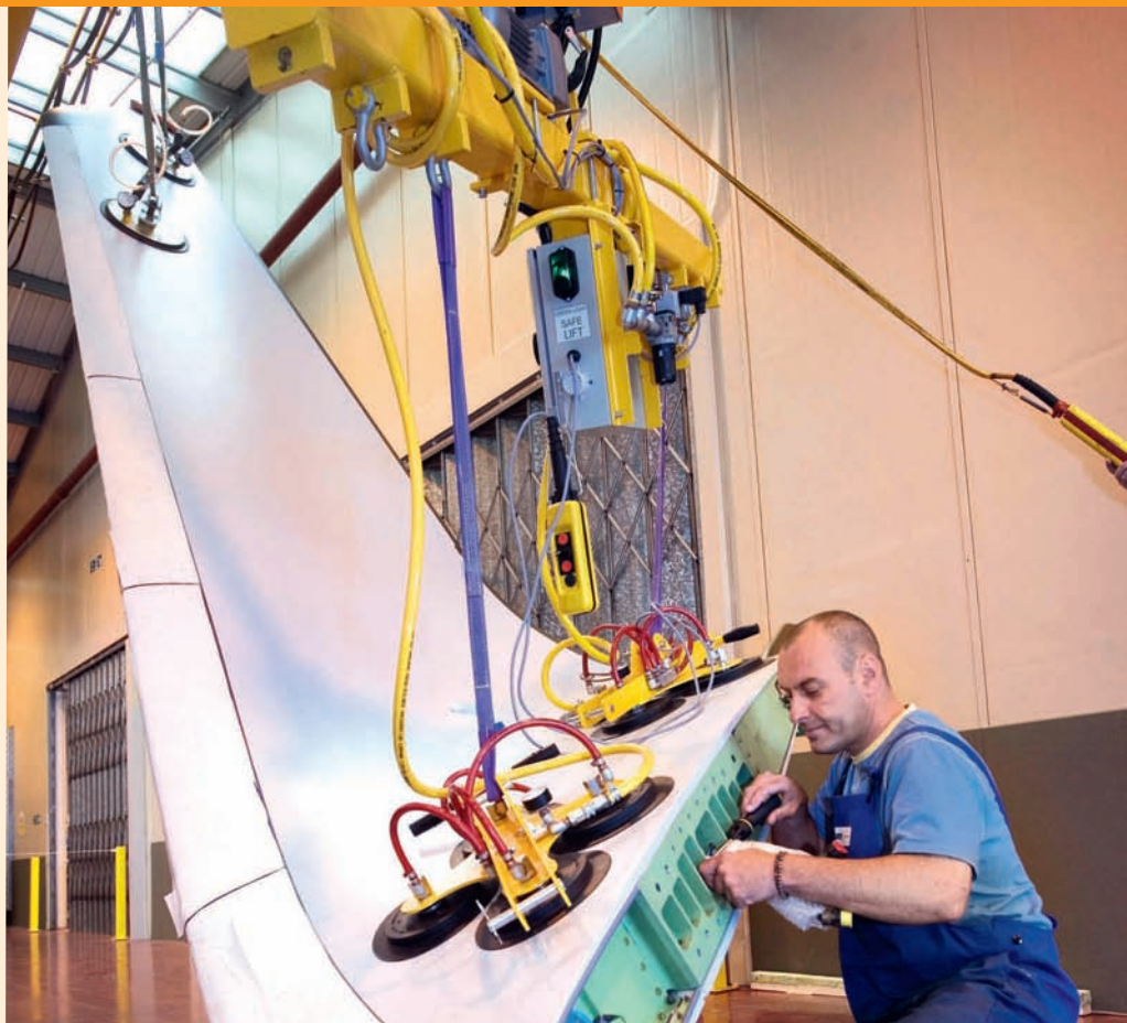
Boeing 767 blended winglet: On the assembly line at GKN Aerospace
